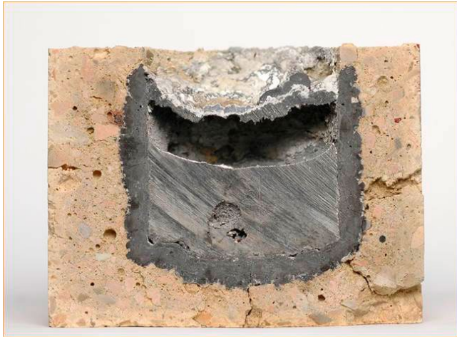
Figure 3 - Cross section showing unreacted refractory with a characteristic T_c . The reacted portion has a new higher T_c affecting about 25% of the total thickness. The net effect is a loss of thermal efficiency.
