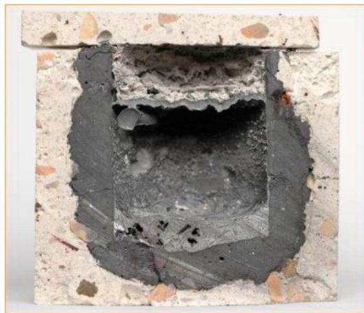
Figure 1 - Cross section of a penetrated and converted Cup Test wall.
