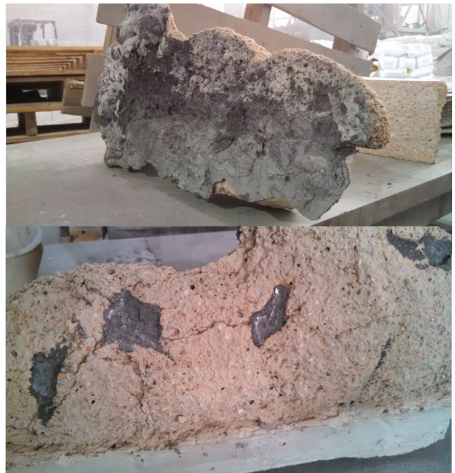
Figure 5 - Section of a used refractory removed from a dosing furnace. The refractory has been damaged and eroded from the cleaning process. The backside is also shown to demonstrate penetration and reaction through cracks and fissures. The freeze plane was in the backup which was penetrated and converted.
