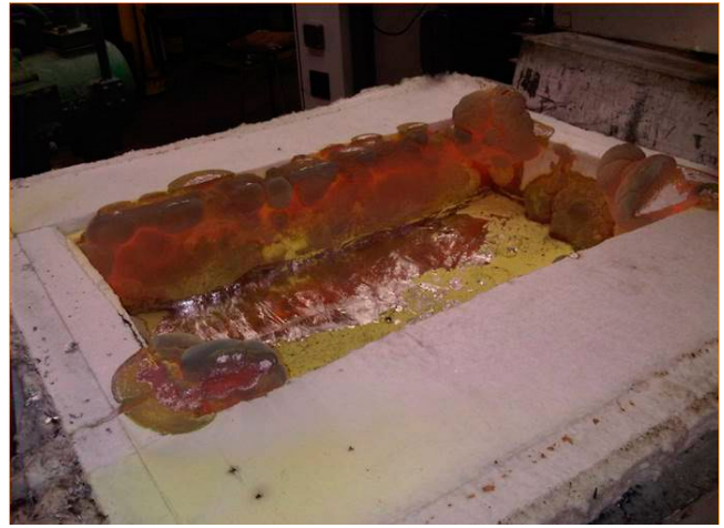
Figure 4 - Small holding furnace with significant penetration, conversion and corundum buildup.
