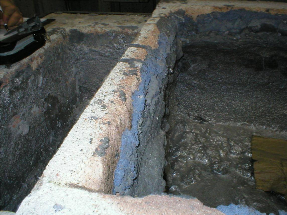
*Fig. 5. Cold Cleaning of DOE-2 Furnace after 1 Year of Service*
