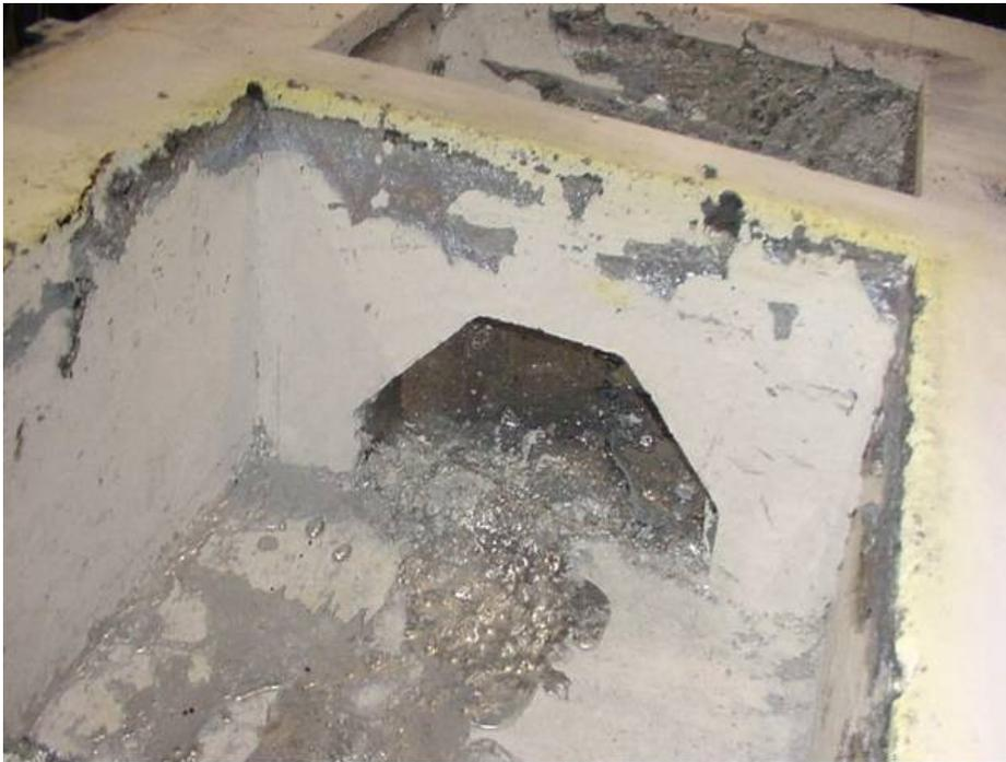
**Fig. 4. Cold Cleaning of DOE-1 Furnace after 1 Year of Service**
