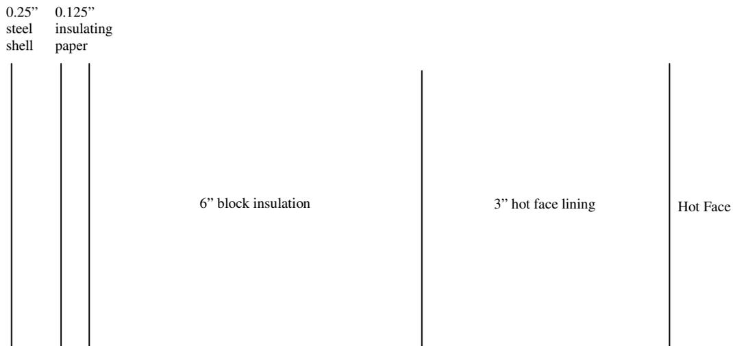
**Fig. 3. Cross-sectional Drawing of the Holding Furnace Lining Configuration**
