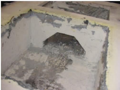
This experiment also demonstrated the much improved performance of formulation D-1 compared to the standard lining after 9 months of service. Figure 5 shows the formulation D-1 furnace after cold cleaning. All material buildup was easily removed from the walls with
