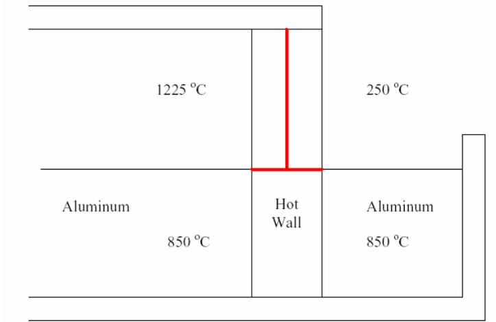
**Figure 8: Hot Wall Temperature Profile**
