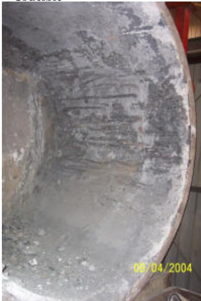
Customer 3 wanted to find a material that would maintain an average insulating character over the lifetime of the crucible, which was an improvement over the current refractory.
