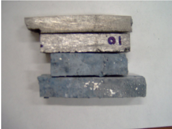
Figure 7. Bars used for MOR testing.
