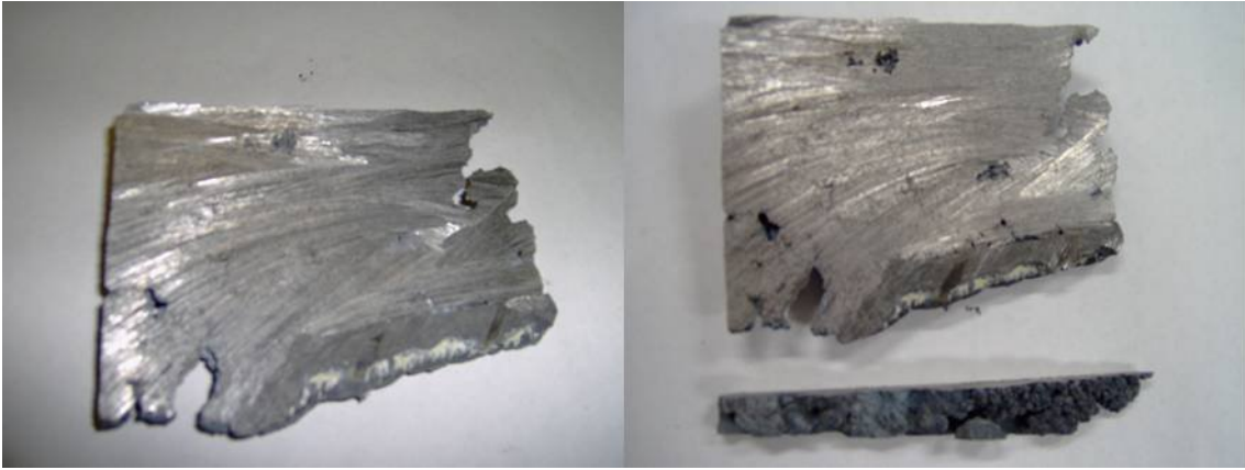
Figure 3. Interior of samples showing metal / oxide mix.
